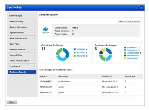
If the Container Security app is already activated and the Container Sensor is not installed on the host, you will be prompted to install the sensor in order to view the vulnerabilities present on the images and containers.
