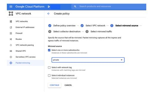
• Select the newly created internal load balancer (forwarding rule) as the destination of packet mirroring.
