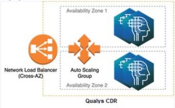
Qualys CDR can be deployed in high availability autoscaling mode using the Terraform module provided for two availability zones (2AZ) and three availability zones (3AZ).
